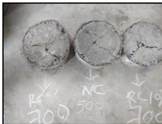
Figure 26: specimens with GFRP sheets after impact test
